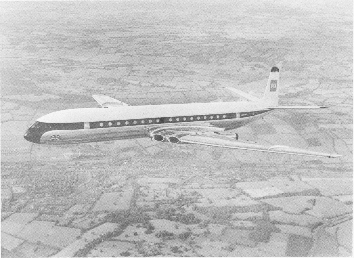
THE DEHAVILLAND COMET 4B, powered by Rolls Royce Avon engines, is shown on a test flight on June 27, 1959. The Comet carries 102 passengers 2500 miles.
